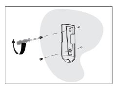
Install the fan remote bracket on the wall as shown.
